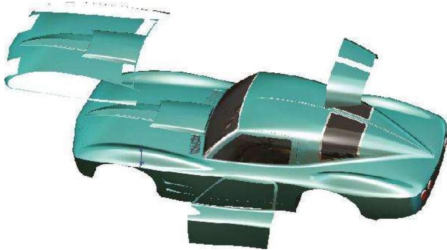
FIGURE 13.5 Pulling parts off of the master model
