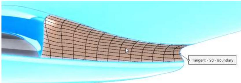
Next, at the tip of the wing, we want to create a little winglet, or curved tip for the wing. Start with a 3D sketch extending the edges of the wing in a natural-looking curvature and distance.
