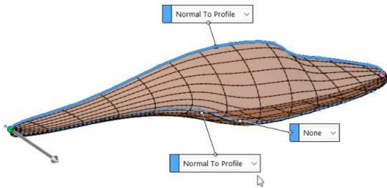
There are several ways to make the wing, depending on what kind of data you are starting from. If this will be a more technical model for you, you can create airfoil curves for various points along the wing and loft together those sections. In this case, I just have two cross sections – the symmetrical point and the wing tip. Both of my sketches are created from two splines – one on the top and one on the bottom. This can actually be tricky.
