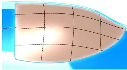
In the back, I used a larger curve, less free form, more controlled, going all the way across. Notice that this one isn't tangent to the sides, but the bulge is more gradual, and more controlled.
