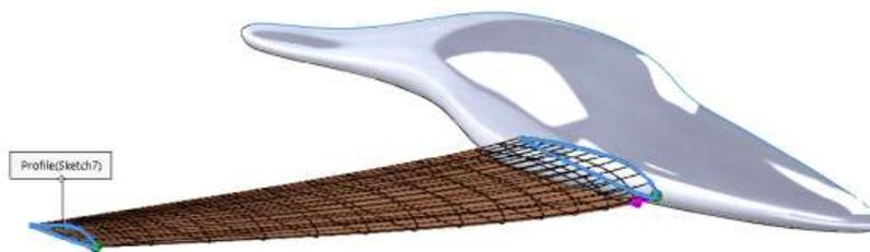
I'm trying to integrate the wing into the fuselage at the bottom to maximize the room inside the fuselage and keep the wing as stiff as possible.
