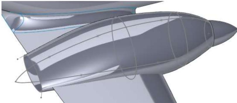
To cap off the engine cowl, since we've been making a lot of degenerate surfaces, I thought we might try to avoid that this once. So here we go with a Fill feature with a constraint curve.
