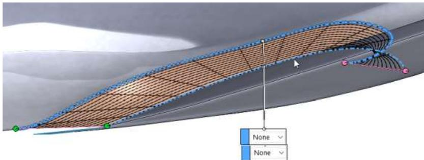
Notice in the image above, on the left side you have two small green dots, and on the right side you have two small pink dots. These are called connectors, and you can use them to straighten out lofts/boundary features, or limit the length of an edge you want to use. In this case, we want to limit the portion of the fuselage edge to use for the blend.
