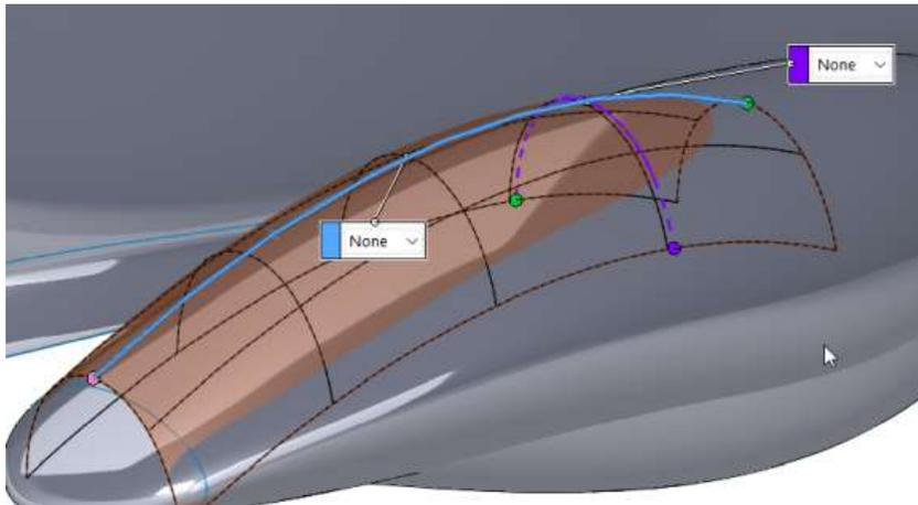
Without getting bogged down in too much detail, I want to move forward into the cockpit area. First we trim out the areas for the glass. I want to add some shape to the glass that isn't in the original fuselage shape. This may be bad for aerodynamics, but I want to show how to use some of these options with the Fill feature.
