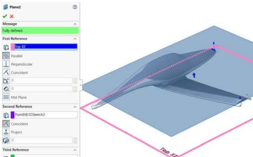
Sketch another airfoil shape on the new plane, and connect leading and trailing edges to the 3D splines. You may need to add a third 3D spline to drive the shape for the wing tip feature properly.
