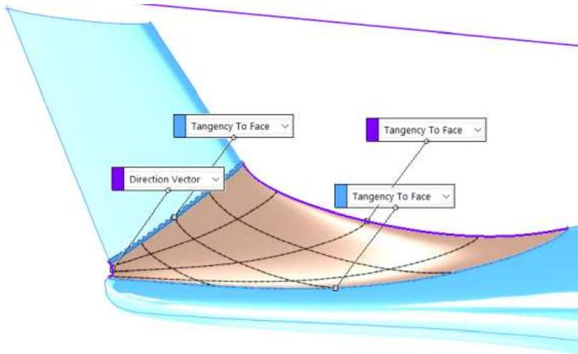
The horizontal surfaces of the tail are created just like the main wing.
