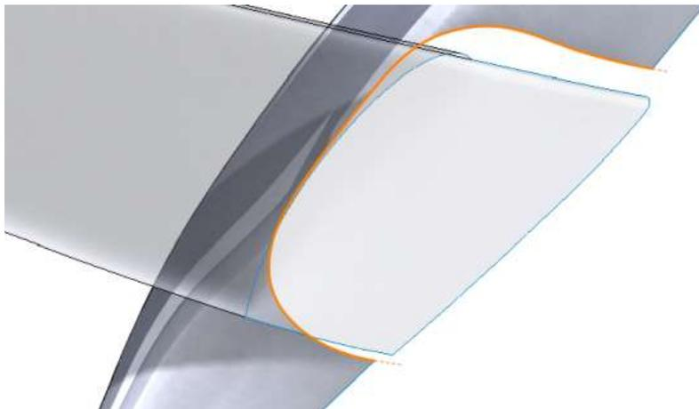
I used one trick after sketching this spline and before trimming the surface. I used Split Entities on it. You can find this at Tools > Sketch Tools > Split Entities. This in effect divides the single spline into multiple splines. It works with other sketch entities as well. I split the 3D spline twice, as shown below, so that the split will create an edge that corresponds to the edge on the wing allowing me to make a blend surface between them.
