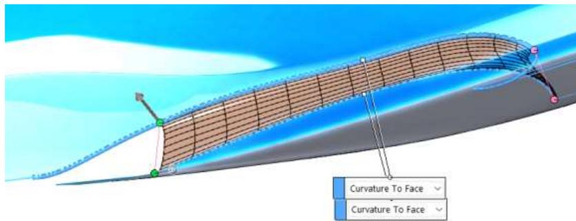
Now you might notice (if you did not use the Split Entities method) that the edge on the fuselage is still a single continuous edge. To make the rest of the blends, you need a front and back area of the fuselage edge. The way to get that is to use Knit to knit the fuselage to the blend surface. So go ahead and do that.
