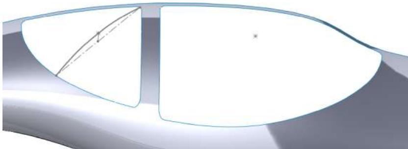
You could choose to set up these 3D sketches before you trim out the cockpit areas, or not. To get good with 3D surfaces and visualization, you have to have a good grasp on 3D sketching, even freehand 3D sketching.
