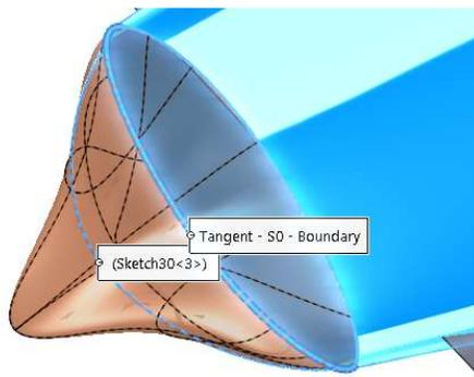
I tried the Fill surface with a 3D sketch point as the constraint, and then a 2D sketch point. Neither one worked. Without a constraint curve at all, it worked, but it didn't do what I wanted it to do.
