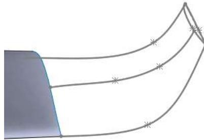
Create a new Boundary surface to merge the wing tip with the rest of the wing smoothly.
