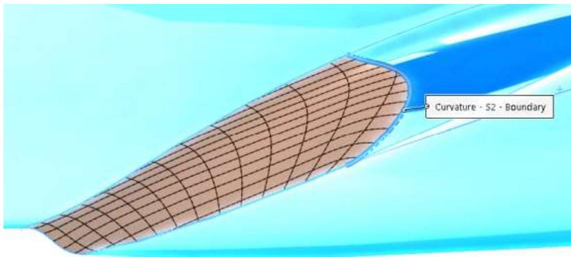
You can do the same sort of procedure to fill in the blend area in the front of the wing.
