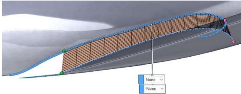
And next apply the Curvature condition to both edges. (If the tangency/curvature goes the wrong direction, use the black/white arrow symbol to flip the direction).
