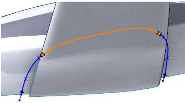
The Split Entities splits can be removed by just clicking on the point where the two splines meet and pressing Delete. The two splines will merge. If you delete both split points, you get the original single 3D spline back.
