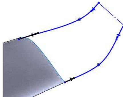
Doing this in a 3D sketch can be hard to judge, so create reference geometry and dimensions where ever you can or need to. Draw both splines in a single 3D sketch, and use the construction line to align the points along the Z axis.
