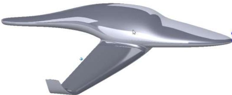
The next step is to attach the tail. The orange sketch below was used to trim out part of the fuselage to fit the tail. The upright tail section was created from a sketch layout, and then a couple of planes, more sketches, and a loft. At this point you should be able to
