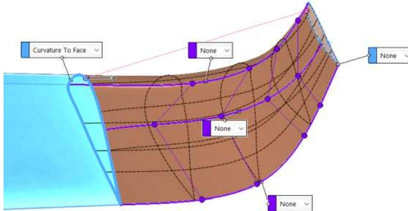
Then to cover the end of the wing tip, create a 3D spline that goes from leading edge to trailing edge and creates a little mound over the opening. Use a Boundary surface to complete the shape. Alternately, you could use a Fill surface here, and avoid another degenerate feature.
