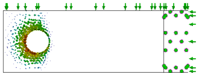
Contact pressure vectors with 1000N force applied
