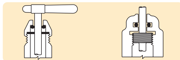
Figure 1-10: Oscillating Seal
