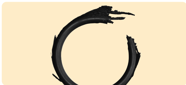
Figure 10-2: Extruded O-Ring
